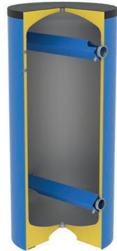
VKR Carbon steel External anti-rust painting Anti-condensate insulation
